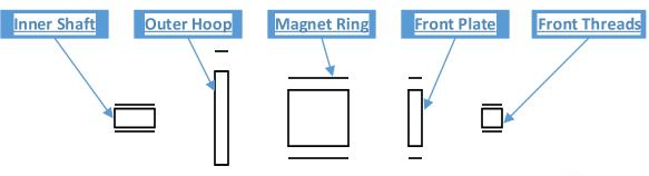
To simplify calculating the Moment of Inertia for the Cosmoneer CMG, we destructively broke it down into five distinct, measurable parts. Since all of the individual parts had holes in the center, we opted for the formula that incorporated the inner and outer radii. With known values in hand, we applied them to the formulas below to arrive at the torque outputs listed.
