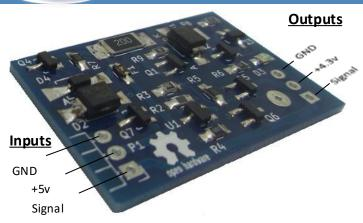
The BRC (Battery Replacement Circuit) fills the role of a battery, providing high current on demand.
