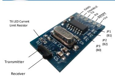
Thank you for purchasing the Serial IrDa Communications Board! In order to use your board you will need a host controller or a USB/FTDI cable with a terminal communications program. You will have greater control of the board using a host controller as the communications software is entirely up to you.
