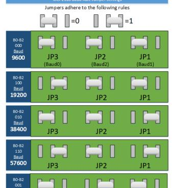
NOTE: Baud rates coincide with a 7.3728Mhz crystal
